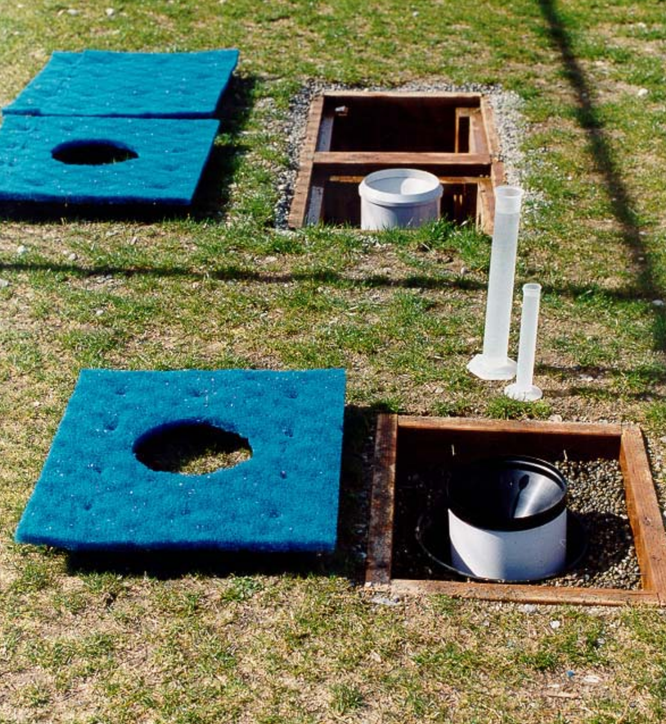
Buried gauges TB3 and Nova Lynx accumulator gauge (foreground) plus furnace filter anti splash system at Viewland Elementary School, Seattle.
