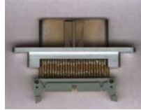
Large thermocouple boundary layer rake Source: http://www.gsc.nasa.gov/WWW/RT2000/5000/585/5hwang.html
