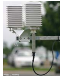
Fig. 4-15 Extreme radiation error in a Gill multiple shield.
