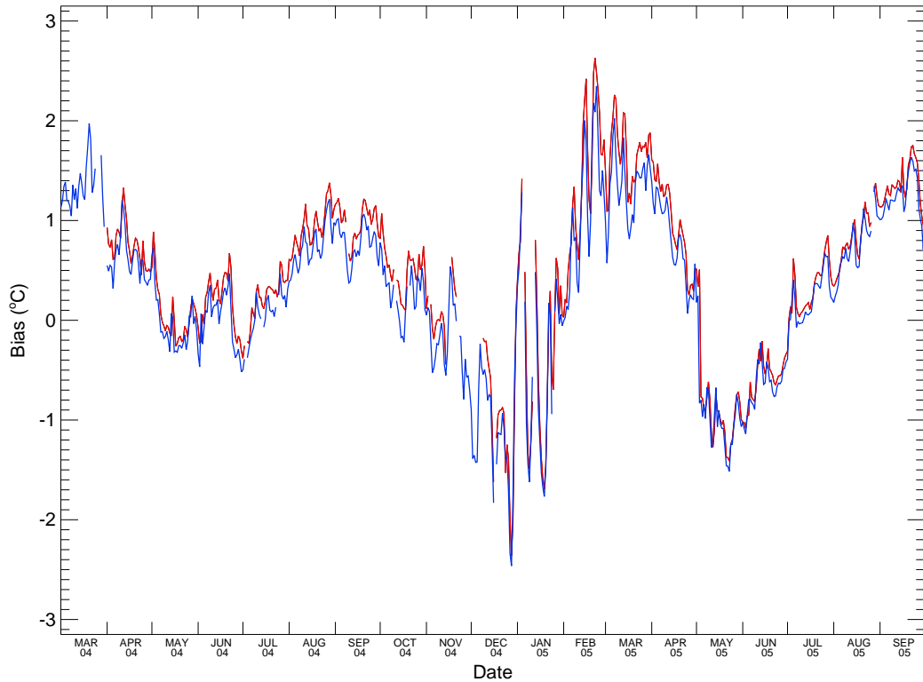
FIG. 4.4: Point calculations of daily soil temperature bias ( ^{\circ}\text{C} ) averaged over all of Oklahoma in the 10–40 cm layer from 0000 UTC (red) and 1200 UTC (blue) Eta analyses compared with 30-cm soil temperature observations from the Oklahoma Mesonet.
